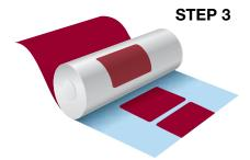
2nd cut is aligned; die advances; material moves forward as shuttle moves forward
