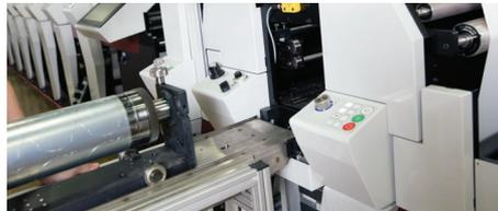
**QCDC** - Also available in semi-rotary, this technology removes the bottleneck of long die changeovers and slower matrix stripping speeds. Available to all Performance Series E models.
