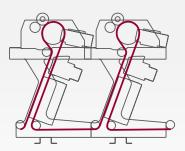
Efficient web path for maximizing both hot air and UV chilled or non-chill applications. No re-webbing needed.
