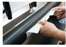
Plate and Tape Demounting Remove plate first, then remove the tape slowly at a flat angle.
