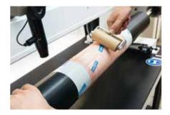
Mount plate with rubber roller, at least on the leading and trailing edge. This will give a better bond than just by hand.
